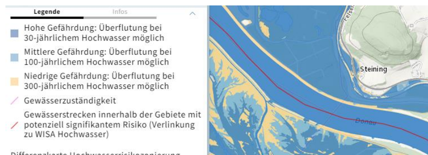
Figure 14: Second example of a view on flood risk which uses the frequency of events to define the score. 35
